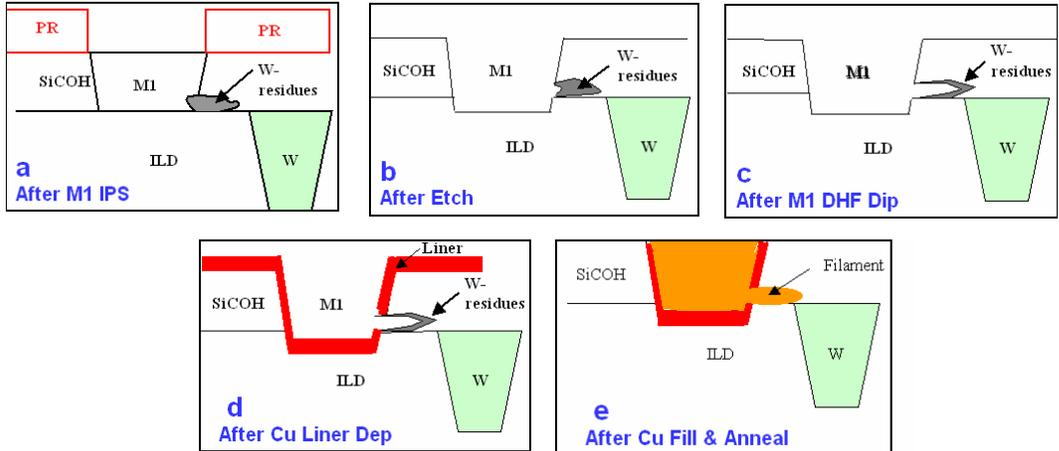
**Figure 6.** Schematic showing the hypothesis of CA induced M1 shorts. a) Residues from W CMP affect M1 patterning. b) Etch rate between SiCOH & residues could be different, inducing notch on sidewall. c) After wet clean, notch was aggravated. d) Liner unable to deposit on the notch. e) Cu will diffuse through the notch, and formed M1 filament.
