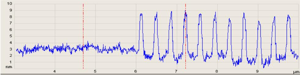
**Figure 7.** AFM profile scanned across contact area after platen 3 W CMP new recipe. It shows that W plugs protruded < 100 Å, which is much more less than that in Figure 4.
