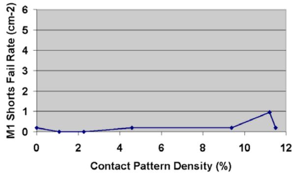
**Figure 8.** M1 shorts failure rate is greatly reduced and independent of contact pattern density with optimized platen 3 polishing time and DI water buff time.
