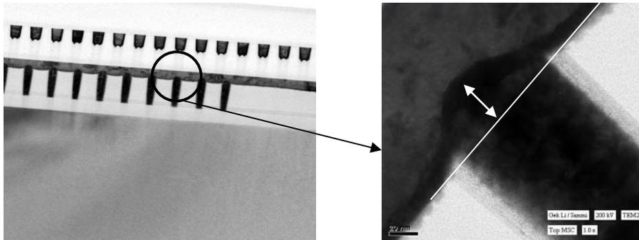
**Figure 5.** Cross-section TEM shows W plug protruded  $383\text{\AA}$ , which has high chance of trapping W-residues.
