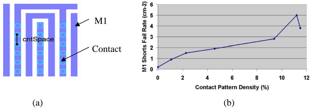
**Figure 2.** (a) Snake-comb structure designed in CV® test chip with contact pattern underneath M1. (b) M1 electrical data shows M1 shorts increased with contact pattern density.
