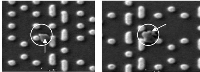
**Figure 4.** SEM scan picture showing W-residues trapped in between W plugs.
