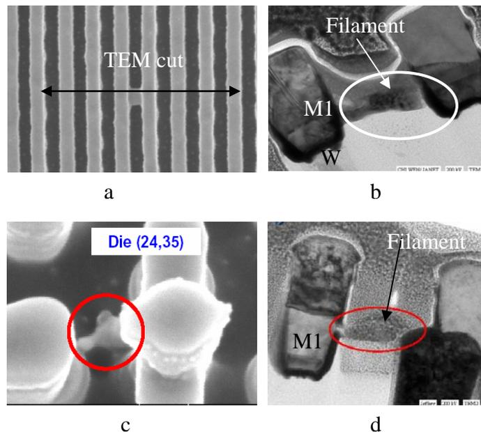
**Figure 3.** a) SEM top -view on M1 to M1 shorts, b) TEM cross-section showing M1 to M1 shorts (filament), c) SEM top-view on CA to M1 shorts, d) TEM cross-section indicates CA to M1 shorts.
