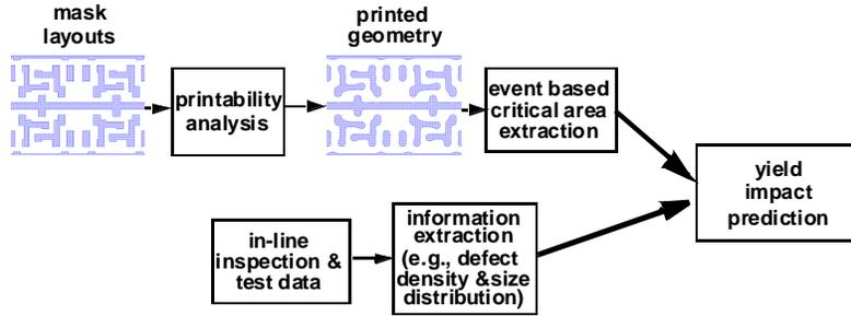
**Figure 1.** Yield impact assessment methodology based on failure event critical area and defect attribute extraction.
