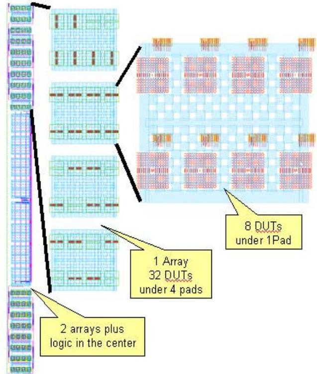
Figure 4: Zoom in from left to right within a layout example of a Device Scribe CV Test Chip.
