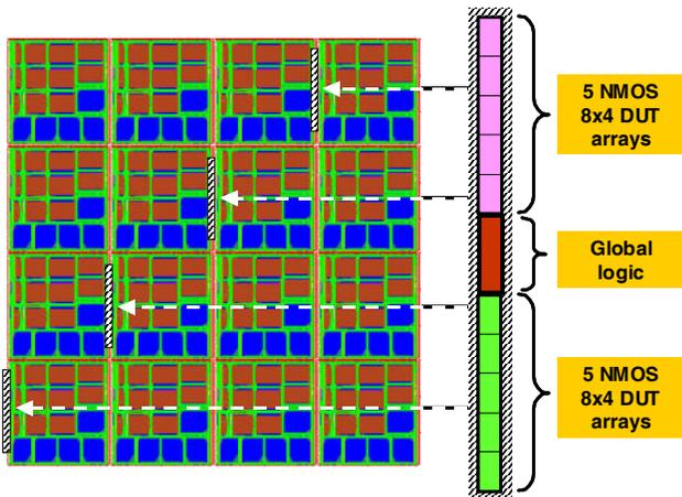
Figure 3: Packing of arrays into one Scribe CV Test Chip (right) and potential placement on a multi-product reticle (left).
