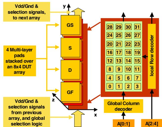
Figure 1: Concept of arranging 32 devices (right) under probe pads (left).
