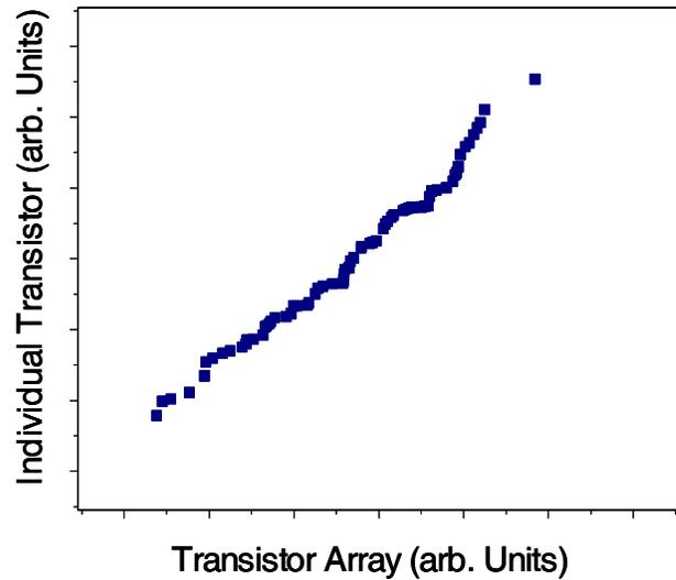
Figure 7: Comparison of Id data from identical transistor layouts taken either from a device array or devices connected straight to the pads.
