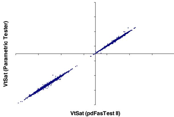
Figure 6: Comparison of Vt measurements taken with pdFasTest II and a standard parametric test system.
