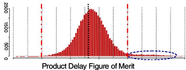
Figure 11: Large sample size of device measurements allows estimation of tails in the performance distribution.
