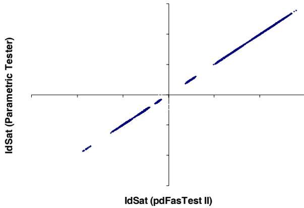
Figure 5: Comparison of Id measurements taken with pdFasTest II and a standard parametric test system.
