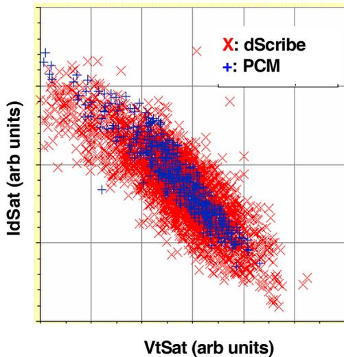
Figure 8: Comparison of dScribe CV measurements with standard PCM measurements from a parametric tester.
