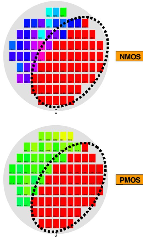
Figure 10: Spatial pattern observed on a set of excursion wafers with a large number of non-functioning devices (NMOS left; PMOS right).
