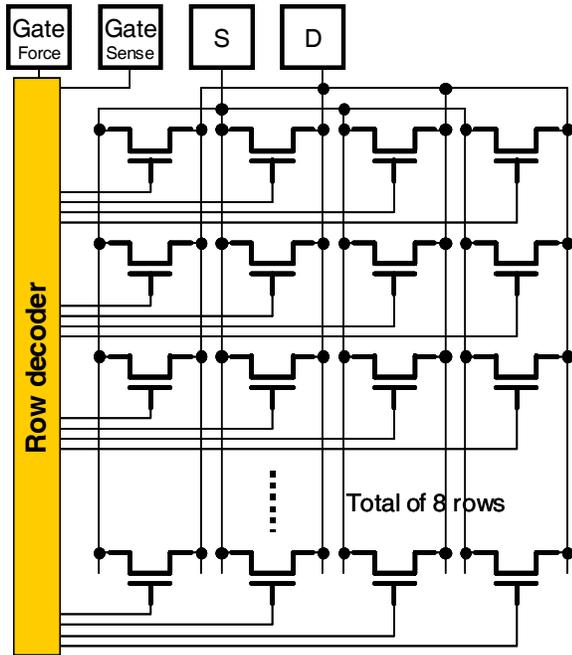
Figure 2: Schematic of one array in the Device Scribe CV test chip.
