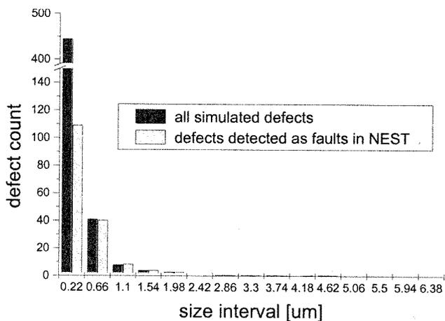
Fig. 9. Comparison of the size distribution of 505 simulated defects and the size distribution of those defects that were detected as faults within a NEST structure.
