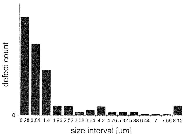
Fig. 12. Size distribution of defects detected within a 0.56- $\mu$ m line pitch (0.28- $\mu$ m line width) NEST structure.
