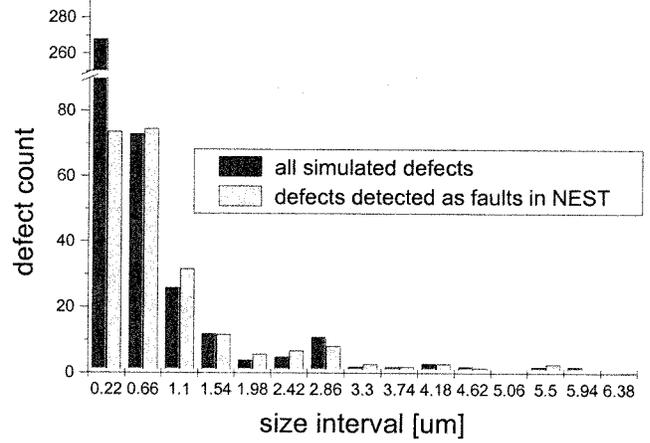
Fig. 8. Comparison of the size distribution of 412 simulated defects and the size distribution of those defects that were detected as faults in a NEST structure.
