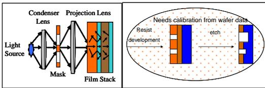
Figure 1. Representation of a typical lithography system on the mask and wafer stack.
