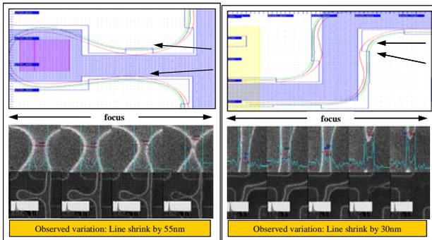
Figure 5. Hotspot examples: T Shape Poly (left) S Shaped Poly (right)
