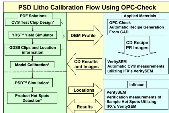
Figure 3. PSD™ Litho Calibration Flow using the AMAT OPC-Check® and VeritySEM™
