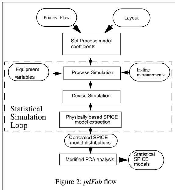
*pdFab* takes as inputs process flow, device layout, and statistical variations associated with the process and equipment. Using this information, *pdFab* generates the physical wafer state (e.g., layer thicknesses and doping profiles), device performance parameters, and physically extracted SPICE model parameters.
