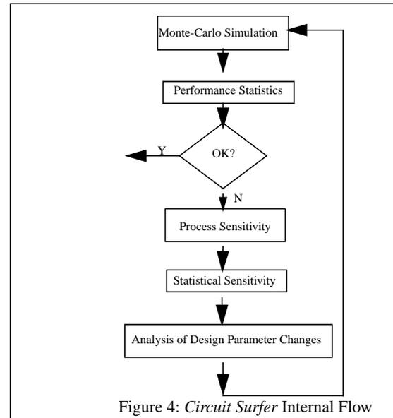
Figure 4: *Circuit Surfer* Internal Flow
