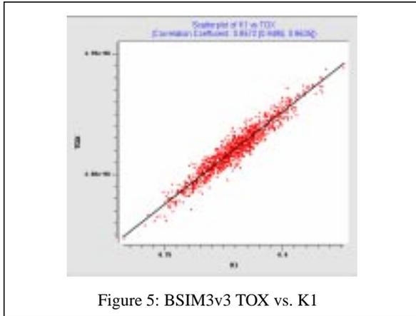
Figure 5: BSIM3v3 TOX vs. K1
