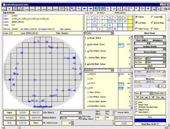
**Figure 2. pdCV software interface for selection of electrical failures. In this example, vias with pitch of 2.73um which did not receive inline defect were chosen for FA.**
