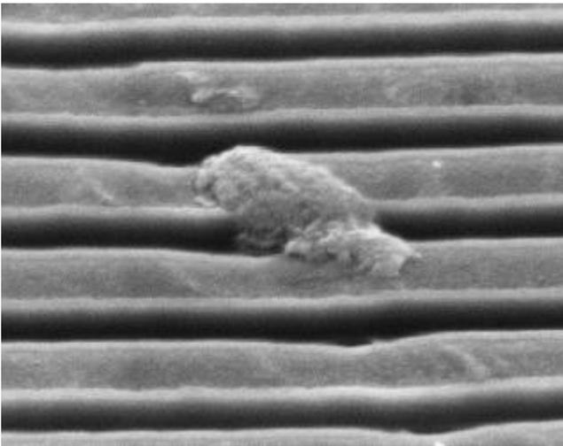
**Figure 6. A shorting defect isolated in a failing structure. This defect can now be cross sectioned and material analysis can be performed immediately.**
