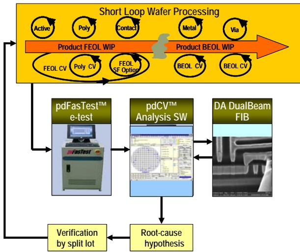
**Figure 1. Methodology for rapid non-visual defect detection and failure analysis with wafer processing flow.**
