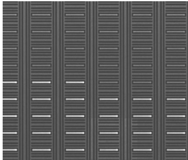
**Figure 3. Top-down view of successful defect localization of a long chain via structure.**
