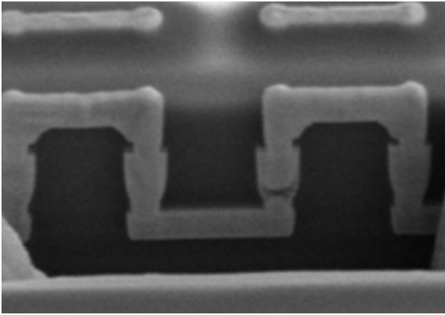
**Figure 5. Dense via chain open. Lower level via has metal void causing structure to fail.**
