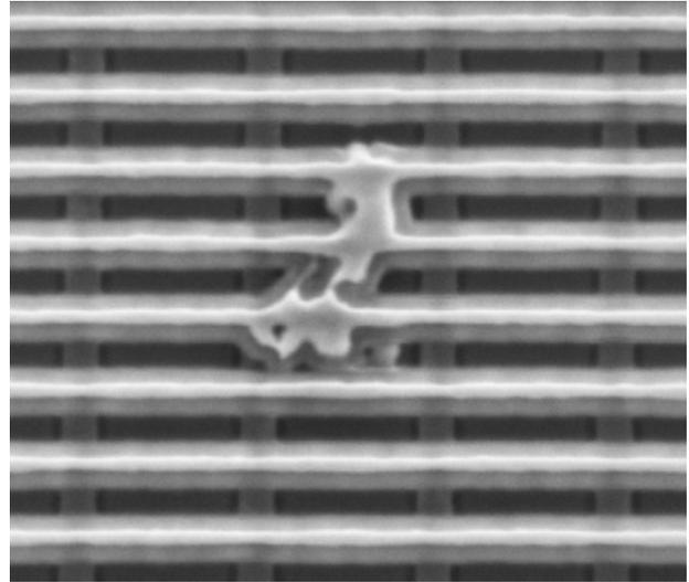
**Figure 7. A poly short defect isolated within a failing structure.**
