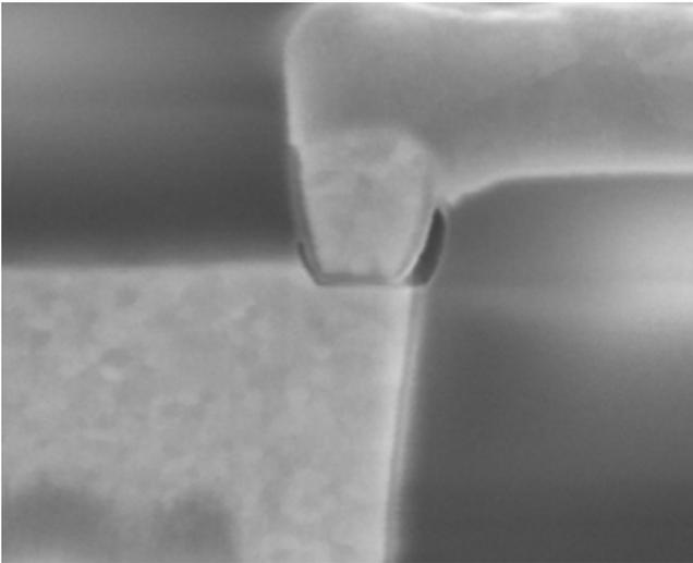
**Figure 8. Contact to local interconnect defect found after FIB cross section was performed.**
