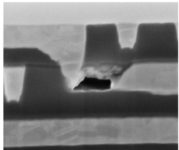
**Figure 4. FIB cross section of large pitch via chain with via open failure.**
