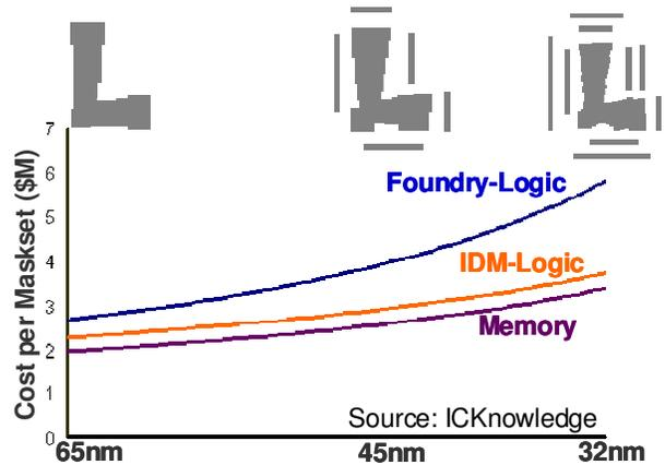
Figure 1: Increasing OPC complexity and mask costs
