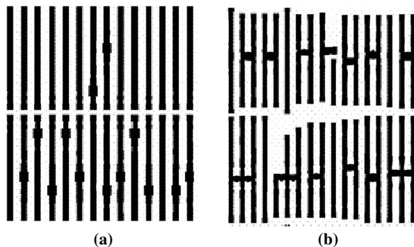
Figure 2: Poly layer model-based OPC (a) pdBRIX (b) Standard Cells
