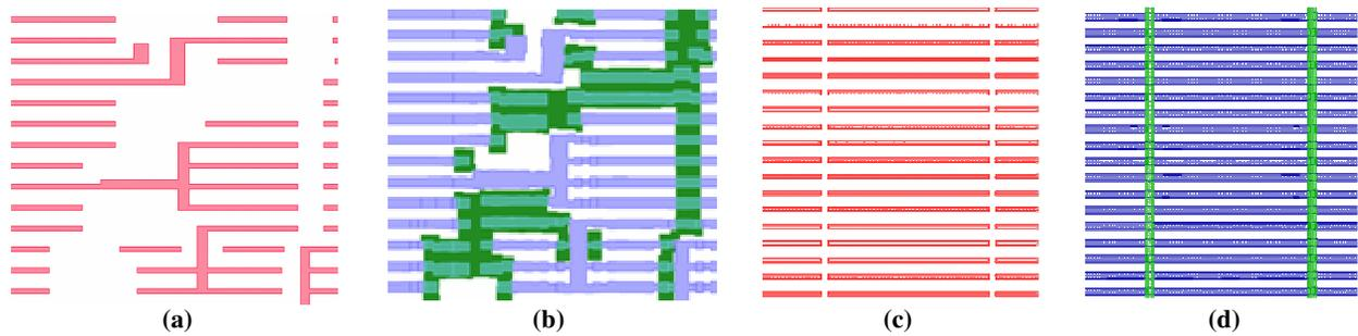
Figure 7: 32nm Poly (a) Standard cell design (b) Standard Cell OPC (c) pdBRIX design (d) pdBRIX OPC
