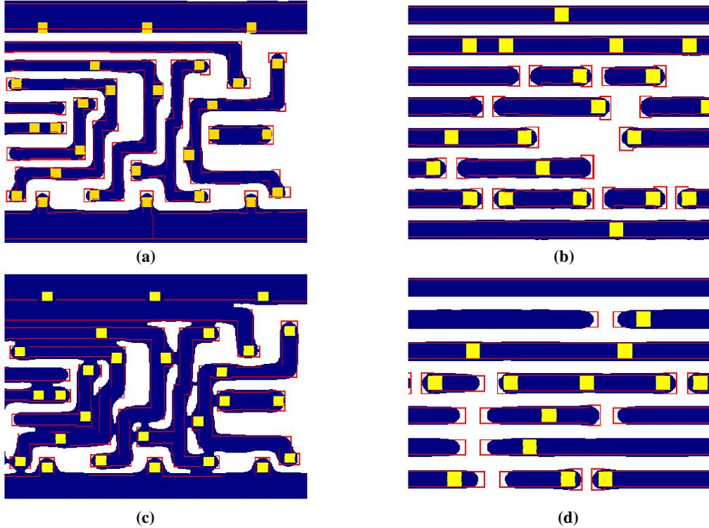
Figure 5: Nominal simulation on 65nm metal 1 (a) Standard cell with model-based OPC (b) pdBRIX with model-based OPC (c) Standard cell with rule-based OPC (d) pdBRIX with rule-based OPC
