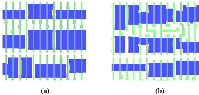
Figure 3: Active layer model-based OPC (a) pdBRIX (b) Standard Cells
